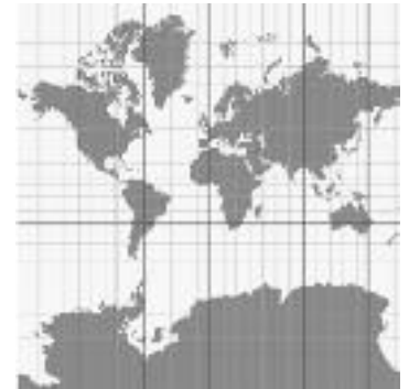
Fig.3: The Mercator projection provides a conformal map of the surface of the earth, so that at any point angles are preserved (but not lengths or areas as can be seen from the over-sized antarctica).
